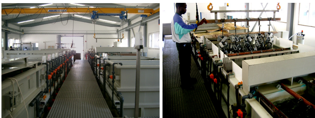
Photo 1 : The anodising baths venue (left) and test parts, just coated
